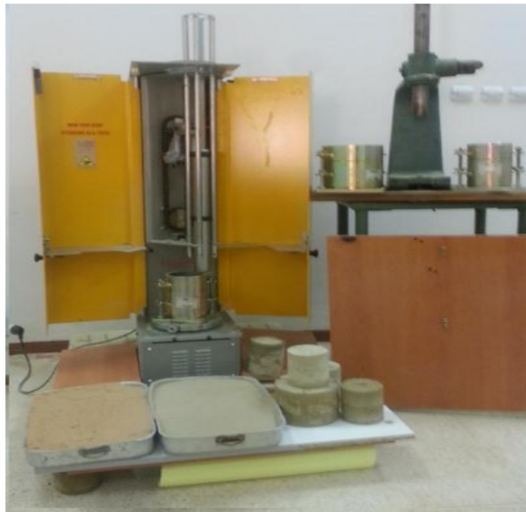
Figure II.8 : Appareil essai Proctor.
